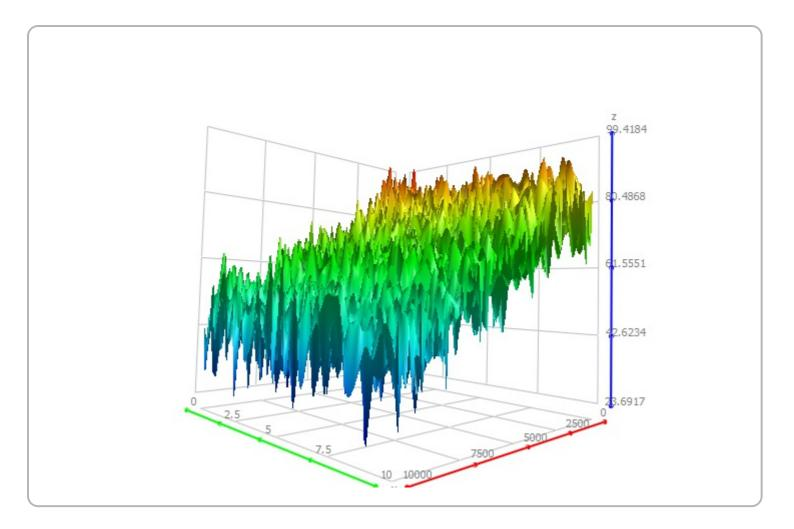
In this example, the engine was revved for a short while during the experiment. The spectrogram shown above illustrates how the dominate frequencies change with time in relation to when the car engine was idle and revved. Using a spectrogram, we can get a deeper analysis of the vibration profile and how it changes with time.
