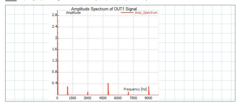
The idea is to use a simple low pass Butterworth filter of the fourth order, with the cutoff frequency equal to 2500Hz. In MatDeck, we can use the IIR form to design the aforementioned filter and to apply the filter to
