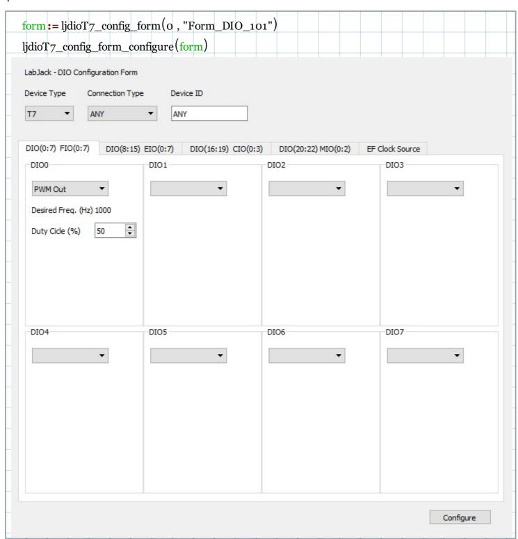
The tab ,EF Clock Source, is used to set the clock source, clock divisor and the roll value for the selected clock. DIO(0:7)-FIO(0:7) is used to set up the PWM output at the selected DIO 0 channel.
