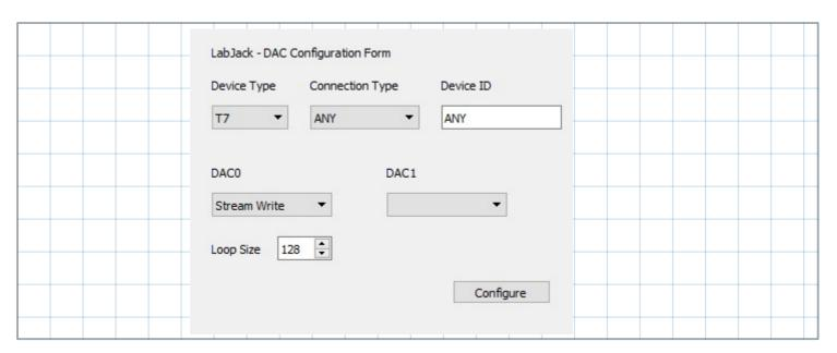
All that is left to do is to set loop values. The device should be opened again as it was closed by the DAC form during configuration.
