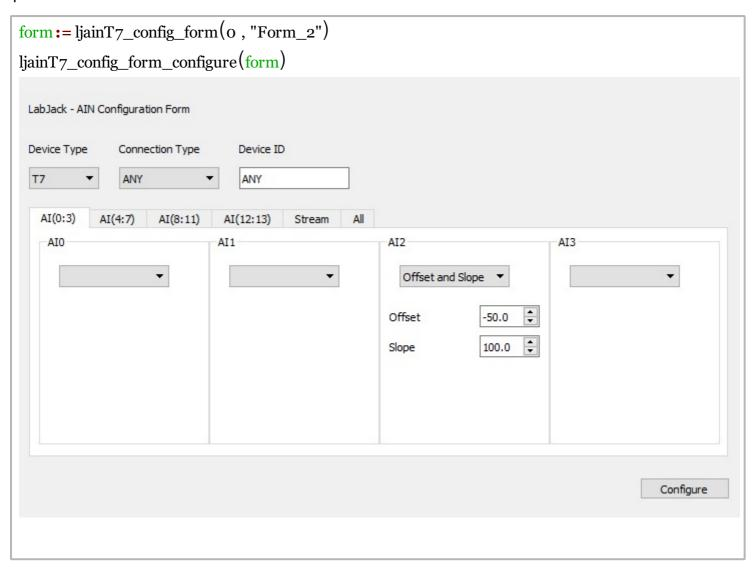
The tab AI(0:3) is used to select extended feature Offset and Slope which is appropriate for this type of temperature measurement. The GUI settings are used instead of script code above..
