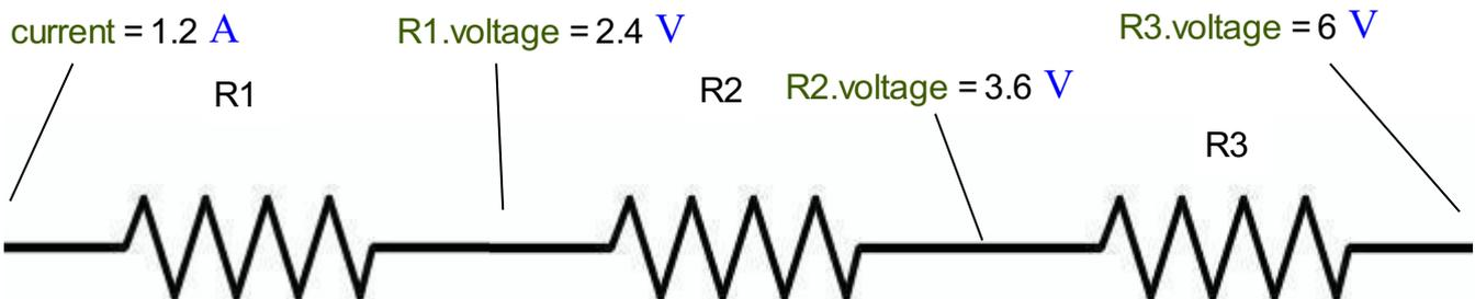
$$R1.voltage + R2.voltage + R3.voltage = 12 \text{ V}$$
