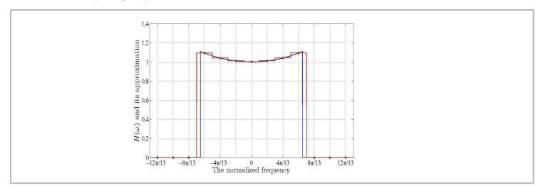
The desired frequency response is sampled at 32 points at regular frequency intervals. Based on the samples of the desired frequency response we can calculate the impulse response of the filter using the following equation.
