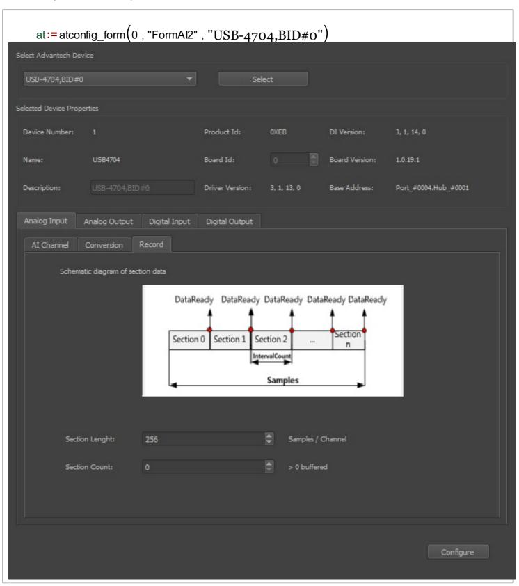
In this example, we use AI in buffered mode, and therefore we only use the aib handle (AI in buffered mode).
